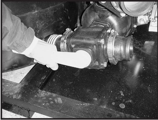
Figure 5.7 Suction Valve Drawing from the Handler
