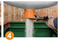
By opening and closing the FLEDBAG you can simply meter the content of the big bag. The slide must be opened towards the body.
