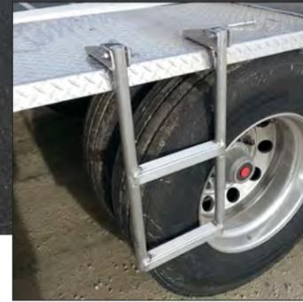
Getting on and off of the trailer easily and safely is important. The Twin Maxx has a hinged aluminum ladder installed onto the fifth wheel platform between the two trailers that is slip resistant and lightweight, yet sturdy and durable.
