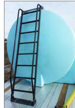
Both of the Twin Maxx's 5,025 US gallon Norwesco tanks have double hinged, slip resistant ladders that, while securely fastened to the tank and the trailer deck, will flex with the trailer during transport. This feature eliminates stress on the tank, trailer and deck common on fixed ladder systems. The powder coated steel ladders also feature a durable adhesive membrane between the ladder and the aluminum deck that prevents corrosion due to diverse metal contact.
