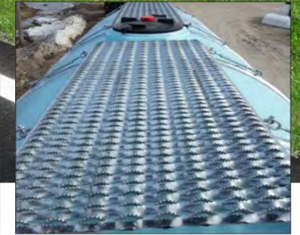
It is important that the access to the tank lid is easy and safe. With a slip resistant aluminum grate custom fabricated from SAFETY-GRIP® Channel, the Twin Maxx platform is securely attached to the support bands and makes for safe access to the top of the tank.
