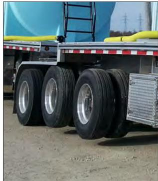
Optional\* individually controlled lift axles can improve fuel efficiency and reduce emissions, prolong tire life, and reduce road damage if raised while the tanks are empty. On rough roads lowering the lift axles when empty can result in reduced bouncing.
