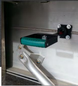
The unique main tank valve is accessible from immediately beside the main plumbing manifold. This valve features an extended valve handle that makes filling and emptying the tank easier than ever.
