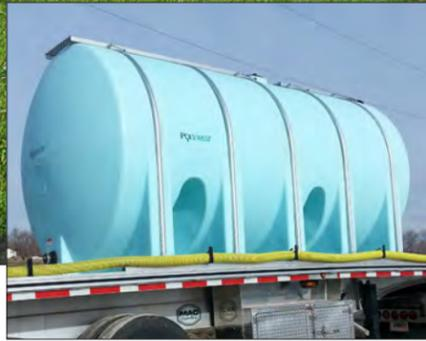
The Twin Maxx includes twin 5,025 US gallon Norwesco horizontal leg tanks built to safely haul liquids up to 1.9 specific gravity. These tanks feature molded-in legs to reduce sloshing with additional liquid movement restricted by Liquid Surge Stabilizer retro-fit baffle balls.
