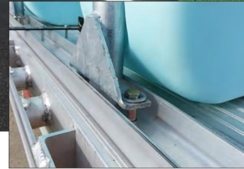
Polywest's own ADFR System is an industry leading method of securing tanks to decks. Designed specifically for the physical characteristics of polyethylene and aluminum, the ADFR System disperses all of the forces inherent in liquid loads to the structural frame of the trailer. This not only provides maximum load security, it also isolates both the trailer deck and the tank from any undue stress and point loading.
