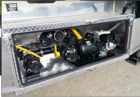
The plumbing system features leak-free Banjo manifold fittings and valves that are vibration resistant and extremely easy to service. The pump options include a 3" Honda-powered Pacer pump complete with the Protec engine protection system or the 3" Honda-powered Banjo pump with a wet seal package to allow for complete run-dry protection. Each trailer has a separate pump and the tanks are designed for either bottom or top loading.
