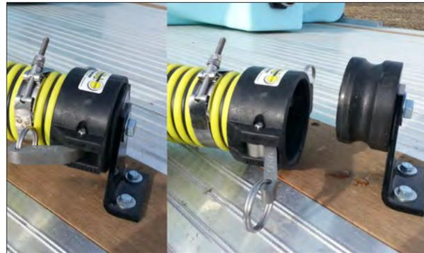
Sometimes it is the little features that save you when you need them the most. The innovative hose management system on the Twin Maxx keeps the 30' of hose supplied with each trailer firmly anchored and sealed during transport, protects the corrosion-resistant polypropylene camlock fittings and provides a safe and convenient area to secure your hose when not in use.
